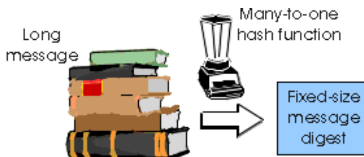
Figure 7.4-2: Hash functions are used to create message digests.
